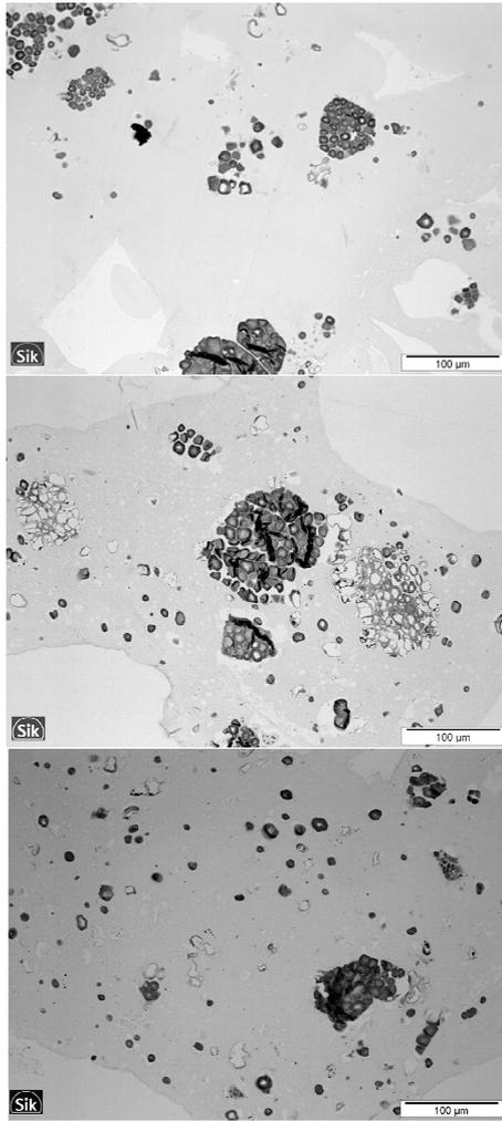
Figure 3. Light micrographs of a reference sample (not foamed, top), specimen 7 (middle) and specimen 9 (below). The protein constitutes the matrix with embedded pearl millet particles.
