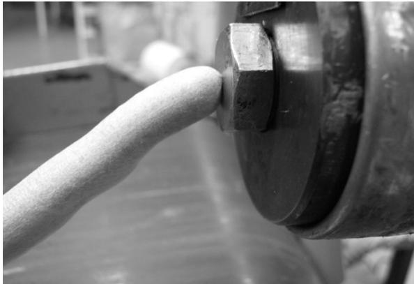
Figure 1. Extrusion foaming of the zein/pearl millet flour blend.
