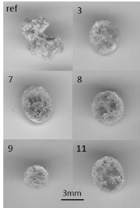
Figure 4. Cross-sections of the reference material (not foamed) and some of the foamed extrudates. The numbers refer to the specimens given in Table 1.
