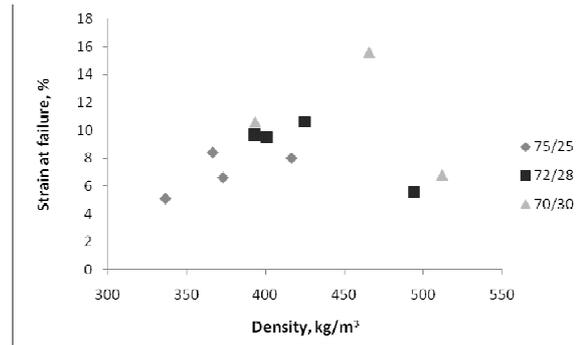
Figure 6. The strain at failure of the foamed specimens as a function of their density. The weight relation between the components (zein/pearl millet flour) is given in the legend.
