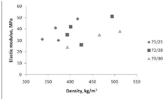
Figure 5. The compressive elastic (Young's) modulus of the foamed specimens as a function of their density. The weight relation between the components (zein/pearl millet flour) is given in the legend.
