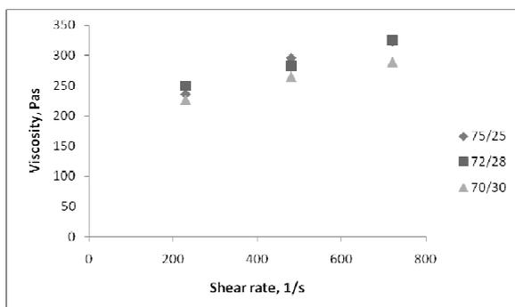
Figure 2. The viscosity of the blends as a function of the shear rate at 90 °C. The weight relation between the components (zein/pearl millet flour) is given in the legend.
