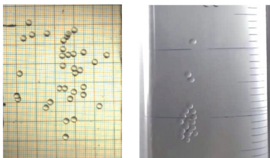
Figure 9. Ensembles of 3mm glass spheres falling spread in water (left) versus (right) as agglomerates in PAC (8g/L).
