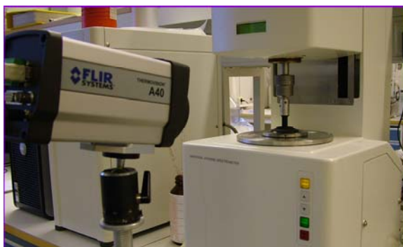
Figure 1: IR camera set-up in front of the Physica UDS200 rheometer.
