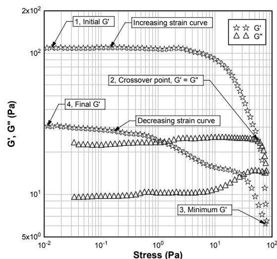
Figure 1. Typical test sequence starting at point 1, increasing the strain to point 2 and 3, then decreasing the strain to point 4.
