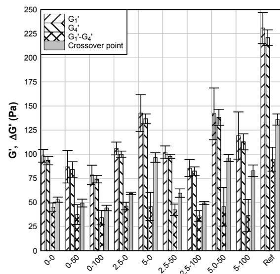
Figure 2.  $G'_1$ ,  $G'_4$ ,  $G'_1 - G'_4$  and  $G'_{\text{Crossover}}$  for the different recipes. The error bars indicate plus/minus 1 standard deviation.
