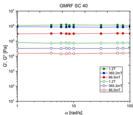
Figure 2. Frequency sweep plot of GMRF SC 40
