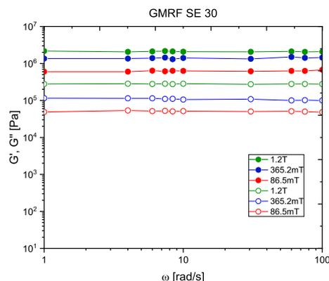
Figure 3. Frequency sweep plot of GMRF SE 30
