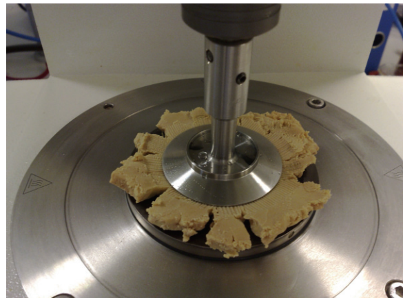
Figure 1: Liver sample prior to removal of excess material. Gap 2 mm.
