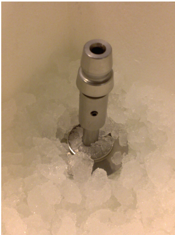
Figure 2: MP31 top plate placed in melting ice.
