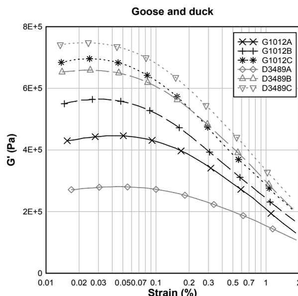
Figure 2. Storage modulus  $G'$  (elastic properties) versus strain for duck- and goose liver at  $+4^{\circ}\text{C}$  using an oscillatory plate-plate rheometer.
