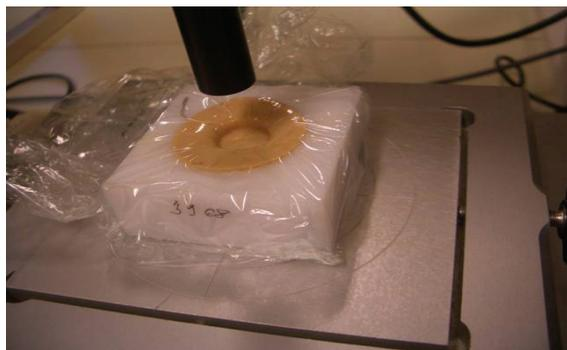
Figure 1. TPA sample covered with plastic film. Probe smaller than sample.
