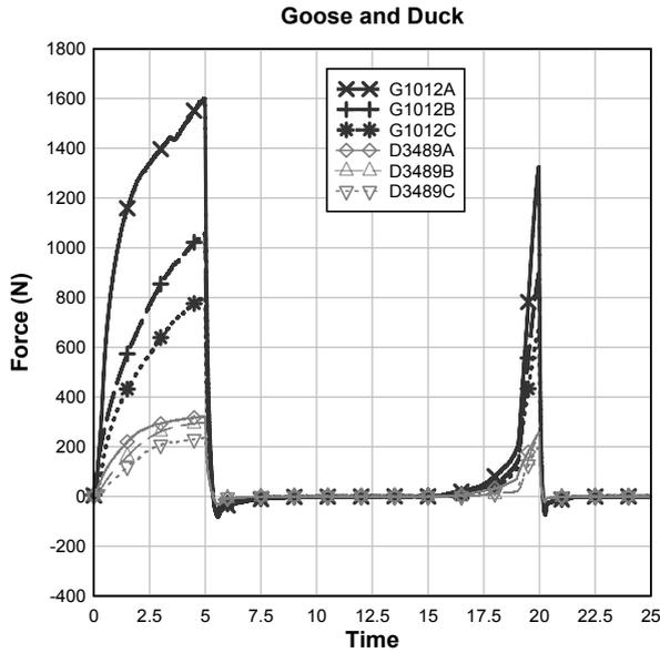
Figure 3. A typical TPA plot highlighting force versus time for one goose - and one duck liver, three two-bite TPA repetitions of each sample at +4°C.
