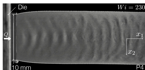
Figure 3. Inline optical extrudate visualization (single frame) of sample P4 at Wi = 230 ( \dot{\gamma}_a = 25 s -1 , n = 65 rpm).
