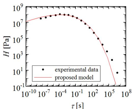
Figure 1. Tentative fit of the proposed model for describing the relaxation time spectrum of bitumen.
