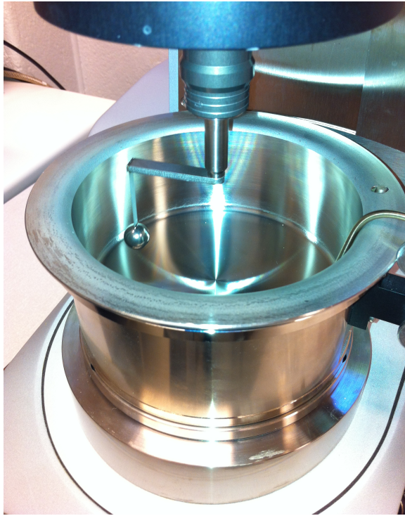
Figure 1. BM 12/72.5 measuring system with an eccentrically positioned 12 mm diameter stainless steel ball.
