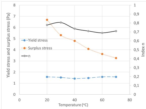
**Figure 9.** The effect of temperature on Herschel-Bulkley parameters  $\tau_y$ ,  $\tau_s$  and  $n$  for the fluid shown in Figure 9.
