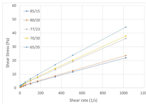
**Figure 2.** The effect of O/W ratio on viscosity at room temperature after 24 hours hot rolling at 90°C.
