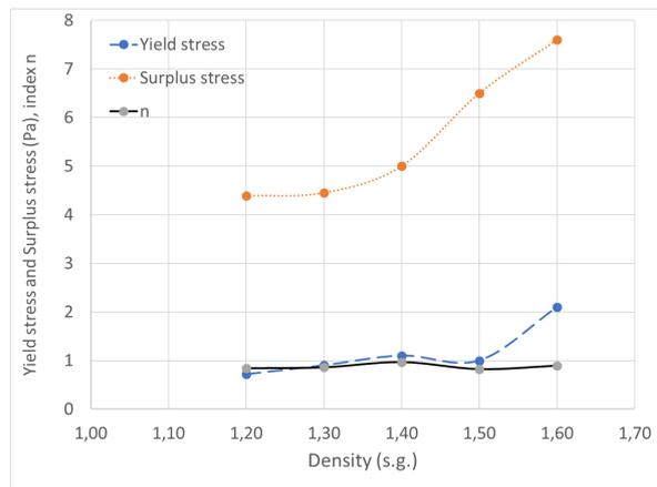
Figure 6. The effect of density on Herschel-Bulkley parameters  $\tau_y$ ,  $\tau_s$  and  $n$ .
