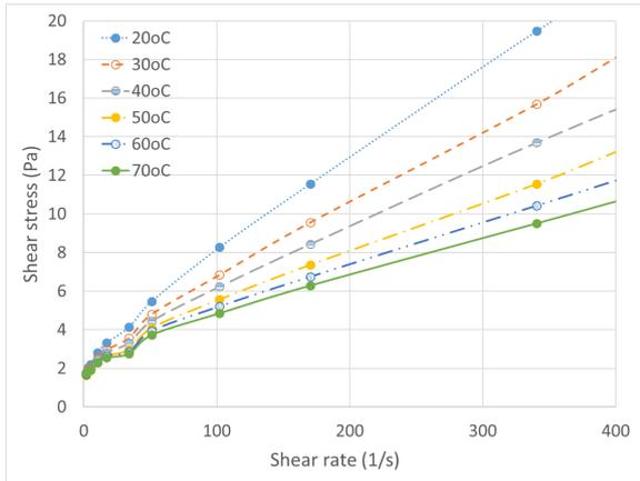
**Figure 8.** The shear stress as function of the shear rate for an oil-based drilling fluid viscosified with organophilic clay at different temperatures.
