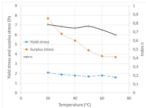
**Figure 11.** The effect of temperature on Herschel-Bulkley parameters  $\tau_y$ ,  $\tau_s$  and  $n$  for the fluid shown in Figure 11.
