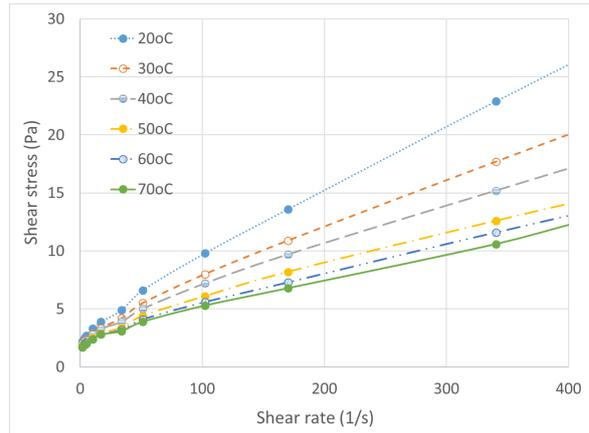
**Figure 10.** The shear stress as function of the shear rate for an oil-based drilling fluid weighted with barite to 1.59 s.g. at different temperatures.
