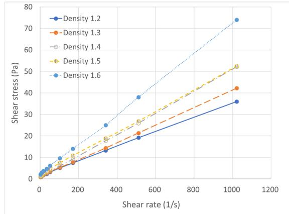
Figure 4. Shear stress plotted as a function of shear rate for five different recipes with increasing barite concentration. Measured after hot rolling.
