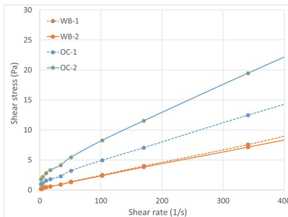
**Figure 7.** The shear stress as function of the shear rate for oil-based drilling fluids with different content of Wyoming bentonite and organophilic clay.
