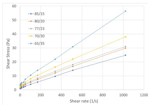
**Figure 1.** The effect of O/W ratio on viscosity at room temperature before hot rolling.
