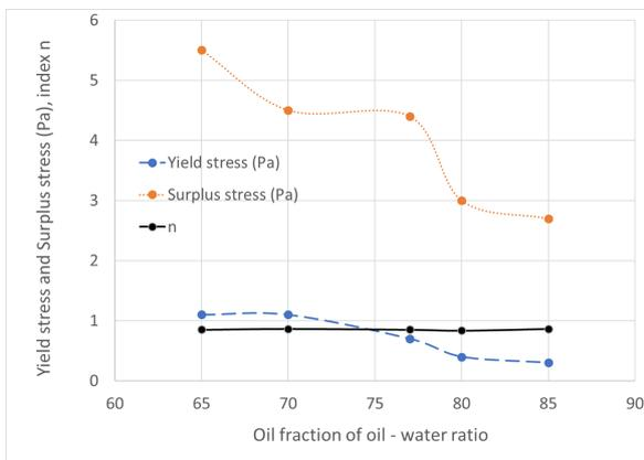
Figure 3. The effect of O/W ratio on Herschel-Bulkley parameters  $\tau_y$ ,  $\tau_s$  and  $n$ .
