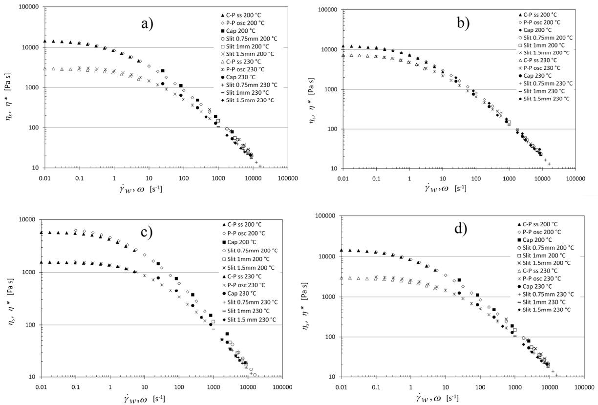
Figure 4. Viscosity curves at 200 and 230 °C a) PP-1, b) PP-2, c) PS-1, d) PS-2
