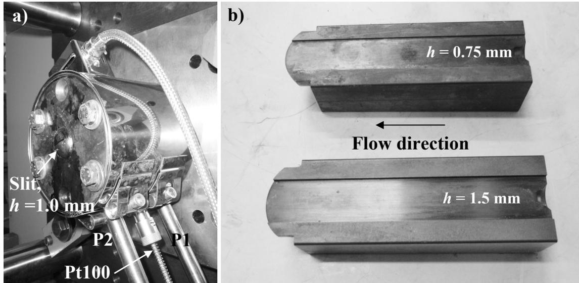
Figure 1. a) The die mounted with 1 mm slit insert, pressure sensors P1 and P2, band heating and temperature regulation with Pt100 sensor. b) 0.75 mm and 1.5 mm exchangeable slit inserts
