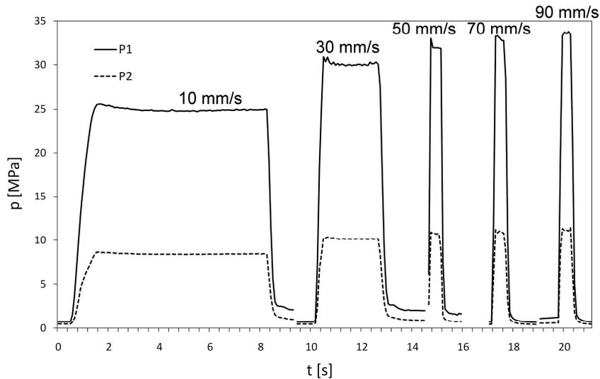
Figure 3. Recorded pressure curves with slit  $h = 1$  mm for PP-2 at 200 °C and injection rates 10, 30, 50, 70 and 90 mm/s. The curves are from separate tests but plotted together to demonstrate the time scale at various injection rates
