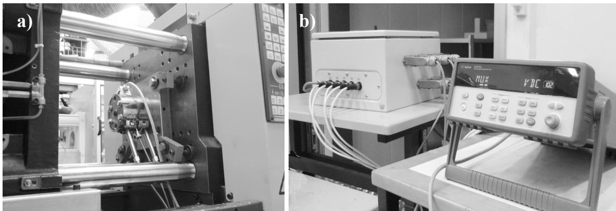
Figure 2. a) Slit die fixed to the mounting plate of the injection molding machine and b) data acquisition equipment
