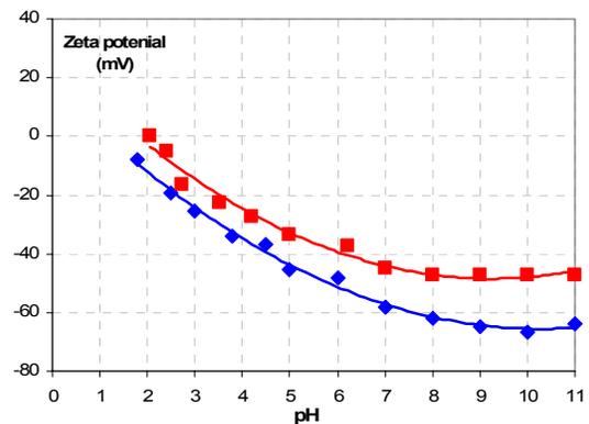
Figure 3. Zeta potential of untreated (■) and plasma treated (◆) carbon fiber samples as a function of the suspension pH in  $10^{-2}$  M KCl.
