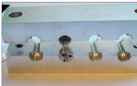
Figure 3. Picture of the steel mould and the new sample fixture.
