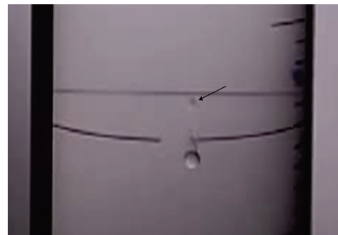
Figure 10: Example of oil drop (shown by the arrow) released from the cavity at 9.16\text{ms} .
