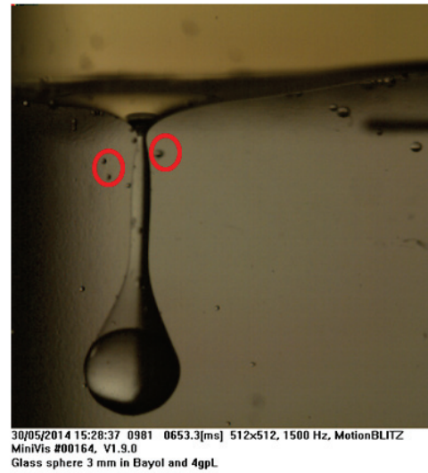
Figure 9: High speed image of the funnel shaped filament attached to the particle. Oil drops are shown (encircled). The image frequency is 1500\text{ Hz} .
