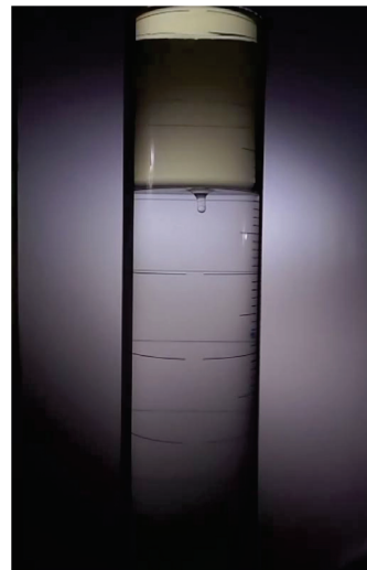
Figure 7: Close up view of the 3 mm glass particle showing the cavitation after crossing the oil phase into the polymer phase.
