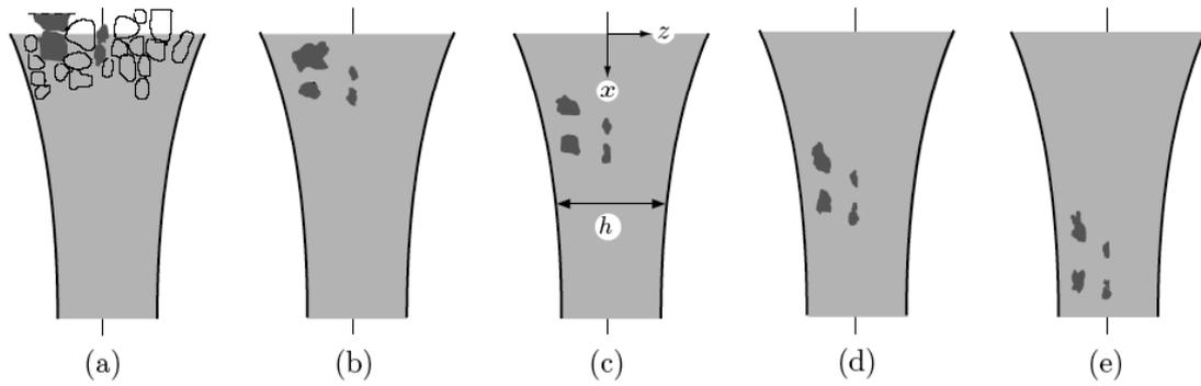
Figure 1. Floc passage through a contraction under technically realistic conditions. Two floc pairs traced out from video frames. Channel y-height 1.3 cm. Linear exit velocity ca. 35 m/s.
