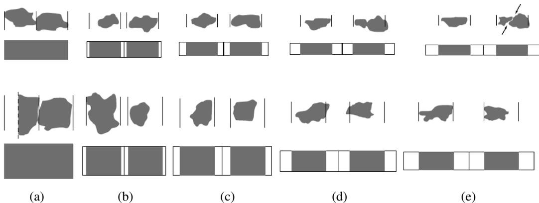
Figure 3. Comparison between experimental and theoretical floc size and floc separation during the passage of the contraction. The series with irregular flocs are copied from Fig. 1. The rectangular modules are circumscribed the flocs in (a) and then developed theoretically.
