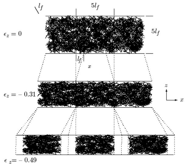
Figure 5. The three-dimensional crunching of a suspended fibre network. Three cubic flocs side by side, with penetrating surface layers of one fibre length are compressed uni-axially just until separation at strain at  $-0.31$ , and then somewhat further.
