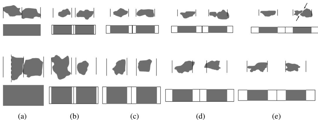
Figure 3. Comparison between experimental and theoretical floc size and floc separation during the passage of the contraction. The series with irregular flocs are copied from Fig. 1. The rectangular modules are circumscribed the flocs in (a) and then developed theoretically.
