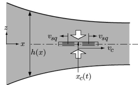
Figure 2. Flow geometry in the contraction with a floc module pair. Floc  $z$ -compression is proportional to the channel height  $h$ .
