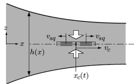
Figure 2. Flow geometry in the contraction with a floc module pair. Floc  $z$ -compression is proportional to the channel height  $h$ .
