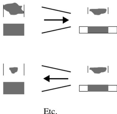
Figure 7. A compression followed by an expansion does not lead back to the initial state.
