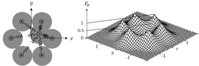
Figure 9. Modelling technical fibre suspension with flocs characterised by loose springs that respond upon compression but separate upon expansion. Central floc movable, the other fixed.
