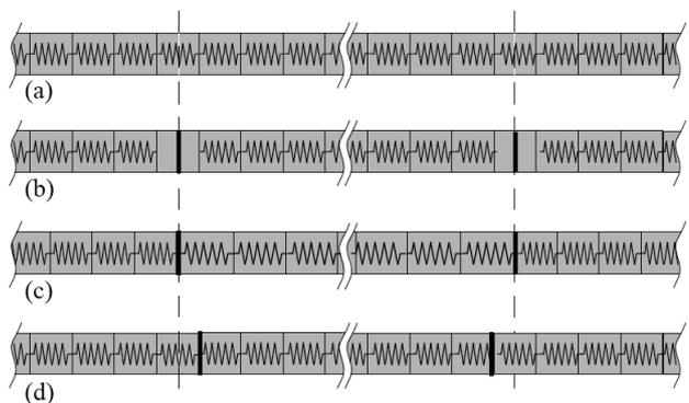
Figure 10. Modelling a compressive stress chain by springs. Separation takes place between the springs.
