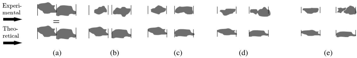
Figure 4. Comparison between experimental and theoretical floc size and floc separation during the passage of the contraction of the small axis-located floc pair. The upper series is experimental. In the lower series, the first floc pair is copied from the first floc pair in the upper series, and has been subjected to theoretical deformations and separated according to the plane squeeze-out model with help of the graphic program (Illustrator).
