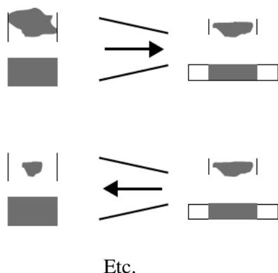
Figure 7. A compression followed by an expansion does not lead back to the initial state.
