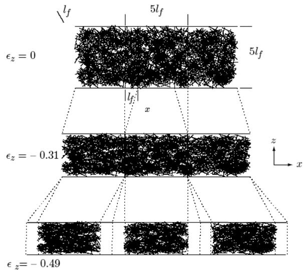
Figure 5. The three-dimensional crunching of a suspended fibre network. Three cubic floes side by side, with penetrating surface layers of one fibre length are compressed uni-axially just until separation at strain at  $-0.31$ , and then somewhat further.
