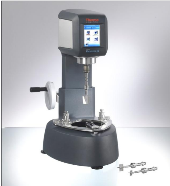
Figure 1. Thermo Scientific HAAKE Viscotester iQ with vane rotor configuration and original container holder.
