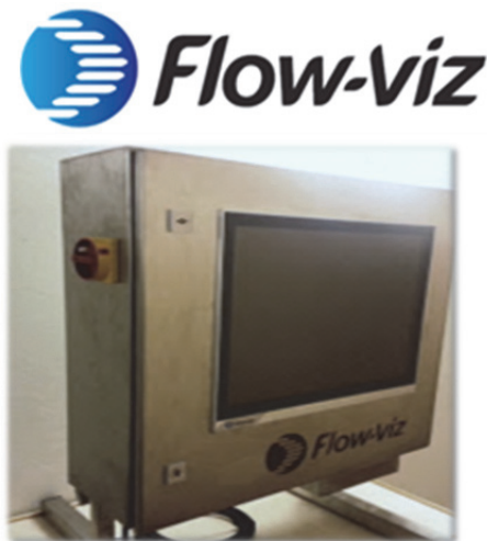
Figure 1. The Flow-Viz operator's panel featuring the electronics, main Industrial PC unit, sensor block and multi-touch monitor.
