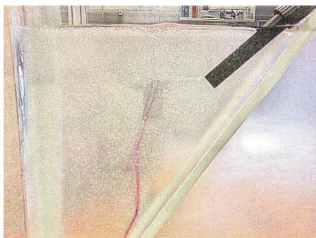
Figure 8. Acoustic streaming in 400 ppm PAC dissolved in water.
