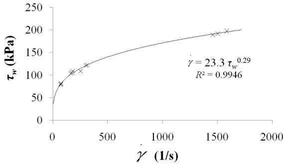
Figure 3. Rheogram for soy dough showing the  $K$  ( $23.3 \text{ Pa s}^n$ ) and  $n$  values ( $0.29$ ).
