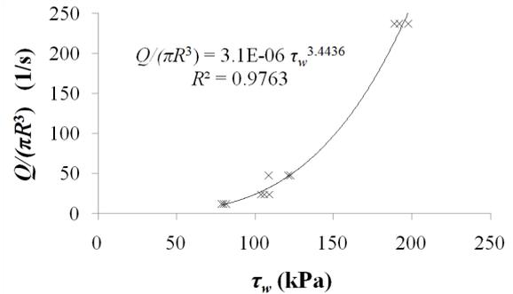
Figure 1. Capillary data for soy dough corrected for pressure loss.
