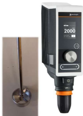
Figure 1. Mixer and blade used in this study for shearing the fluid prior to measuring rheological properties of the fluids.
