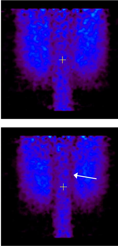
Figure 3. The effect of fraction size on the activity profile. Both images were captured with an upstream velocity of 0.9 m/s fibres acting as the tracers. The upper image represents the case with the R14 fraction as the tracer fibres. The lower image represents the case with the R100 fraction as the tracer fibres.
