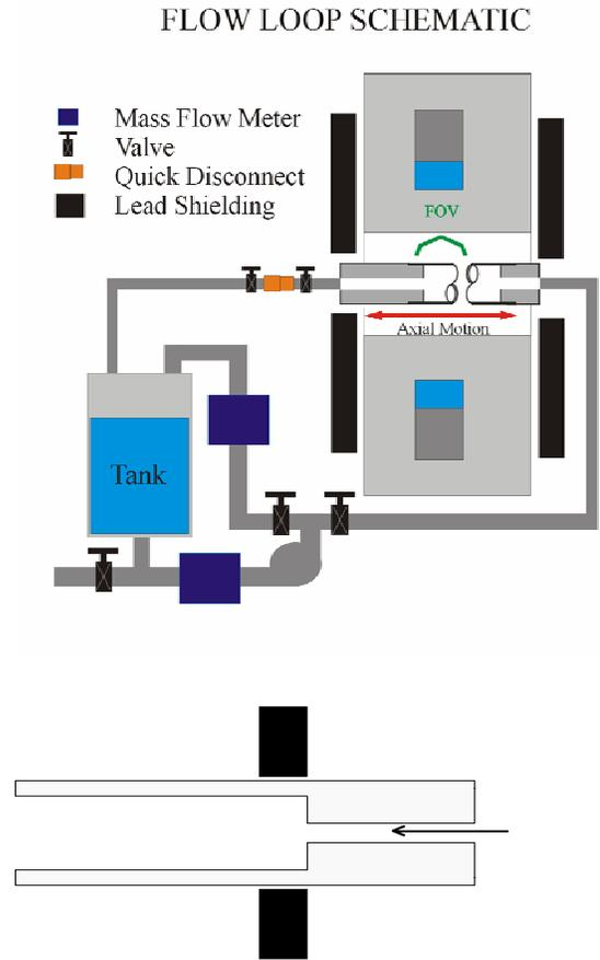
Figure 1. A schematic of the flow loop and the sudden expansion
