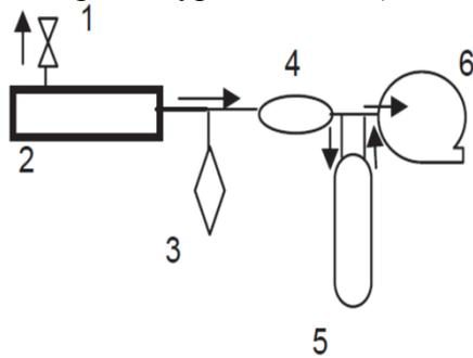
Figure 1. The schematic diagram of the research vacuum moisture removal apparatus: 1-Pressure release valve; 2-Vacuum chamber; 3-Pressure control valve and barometer; 4-Steam condenser; 5-Air filter, 6-Vacuum pump.
