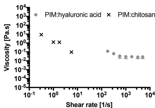
Figure 3. Apparent viscosity as a function of shear rate for mixtures of porcine intestinal mucus (PIM): test sample (v/v). Data is shown as n=3, error bars denotes error propagation.
