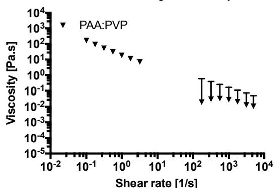
Figure 5. Apparent viscosity as a function of shear rate for mixtures of polyacrylic acid (PAA):test samples (v/v).
