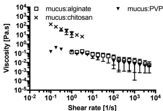
Figure 2. Apparent viscosity as a function of shear rate for mixtures of biosimilar mucus: test samples (v/v). Poly(vinylpyrrolidone): PVP. Data is shown as n=3, error bars denotes error propagation.
