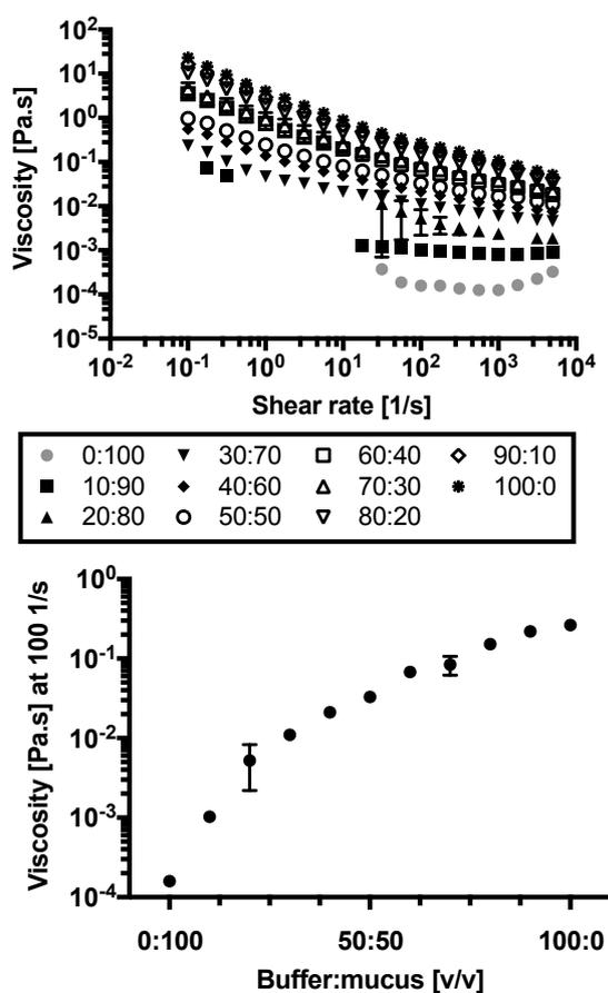
Figure 1. Top: viscosity as a function of shear rate for mixtures of biosimilar mucus:buffer (v/v). Bottom: relationship between dilution of mucus and viscosity at 100 1/s. Data is shown as  $n=3$ , error bars denote standard deviation.
