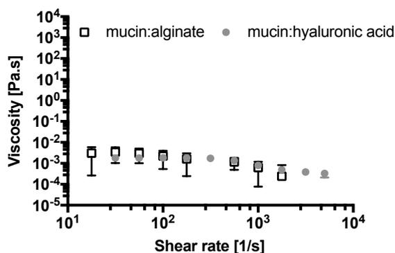
Figure 4. Apparent viscosity as a function of shear rate for mixtures of mucin:test samples (v/v). Data is shown as n=3, error bars denotes error propagation.
