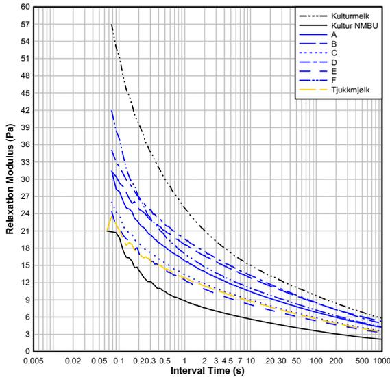
Figure 4. Results from step-strain relaxation tests.
