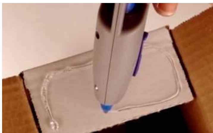
FIGURE 1: Application of the edible HMA using a hot-glue gun.
