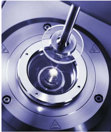
Figure 6. View of the upper and lower measuring plates. The objective with the illumination can be seen underneath the bottom glass plate.
