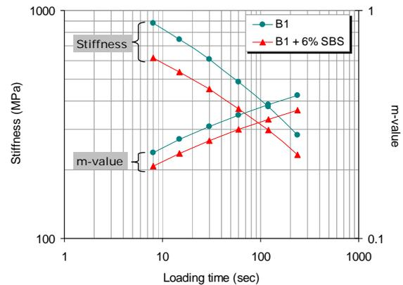
Figure 12. BBR results obtained at -25°C.
