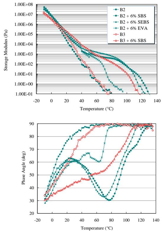
Figure 3. Storage modulus and phase angle versus temperature.
