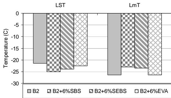
Figure 14. Effect of polymers on the limiting temperatures.
