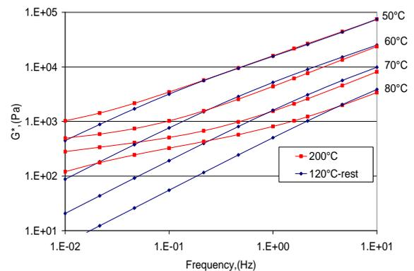
Figure 10. Frequency sweeps for B5+5%SBS.
