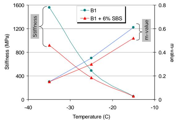
Figure 13. Stiffness and  $m$ -value at a loading time of 60 s versus temperature.
