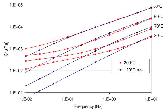
Figure 10. Frequency sweeps for B5+5%SBS.
