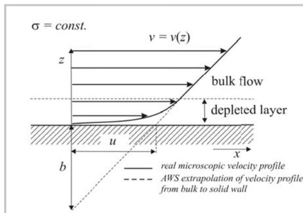
Figure 1. Apparent slip of microdisperse liquid adjacent to a solid wall
