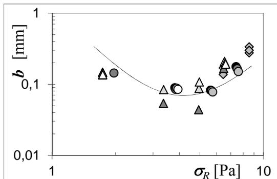
Figure 7. Extrapolated slip length as a function of wall shear stress
