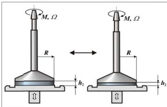
Figure 3. Parallel plate (PP) sensor
