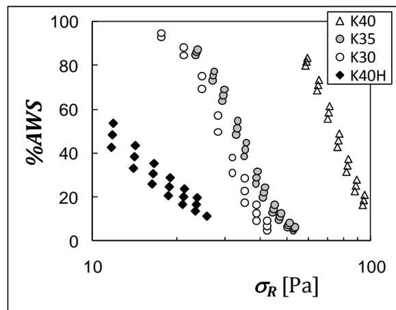
Figure 10. Contribution of AWS to total kinematic effect for kaolin dispersions for the three levels of gap thickness  $h$ .
