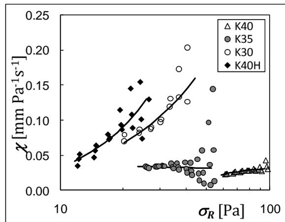
Figure 9. Slip coefficient of the kaolin dispersions.
