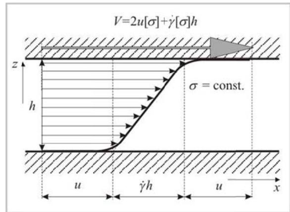
Figure 2. The concept of apparent wall slip velocity  $u$  for the longitudinal flow between two parallel plates (Simple shear prototype)
