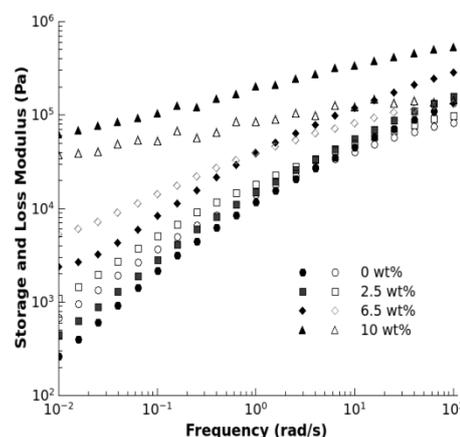
Figure 2. Storage ( $G'$ , filled symbols) and loss ( $G''$ , open symbols) moduli versus angular frequency at 70 °C for the cast PEO nanocomposites.
