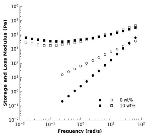
Figure 4. Storage ( $G'$ , filled symbols) and loss ( $G''$ , open symbols) moduli versus angular frequency at 70 °C for extruded nanocomposites with PEG.
