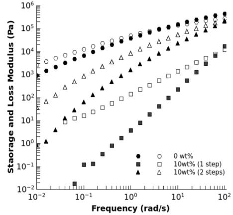
Figure 3. Storage ( $G'$ , filled symbols) and loss ( $G''$ , open symbols) moduli versus angular frequency at 70 °C for extruded nanocomposites with PEO.
