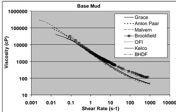
Figure 2. Viscosities of the Base Fluid after a 12% Oil Dilution
