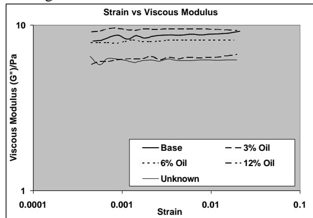
Both graphs show the expected trend of decreasing viscosities as the degree of oil dilution increases with the exception of the smallest oil dilution (3%) where there is a small increase in the modulus in both cases. The percentage change in values for the diluted samples with respect to the base is of the same order as the change in conventional viscosity and on this basis, it does not appear
