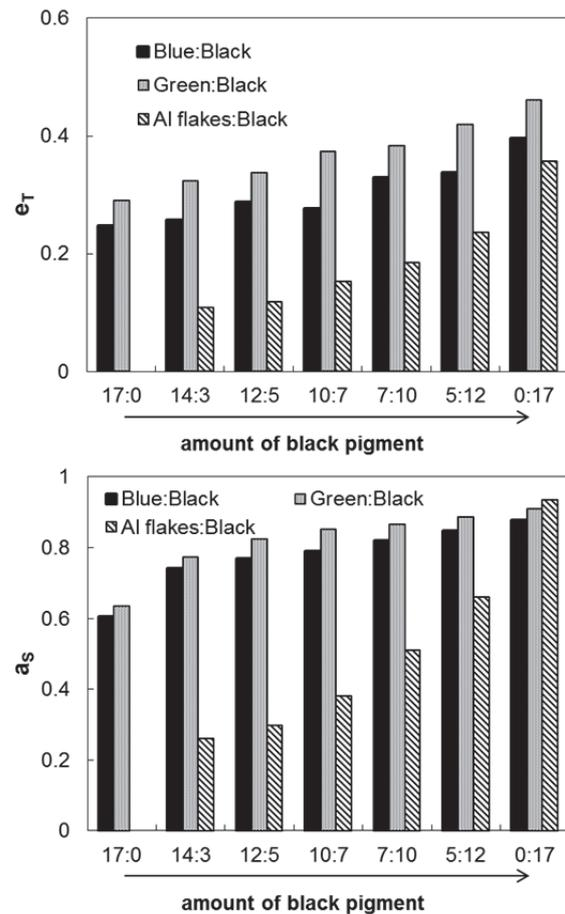
Figure 4. The influence of black pigment on thermal emissivity  $e_T$  and solar absorptivity  $a_S$ .
