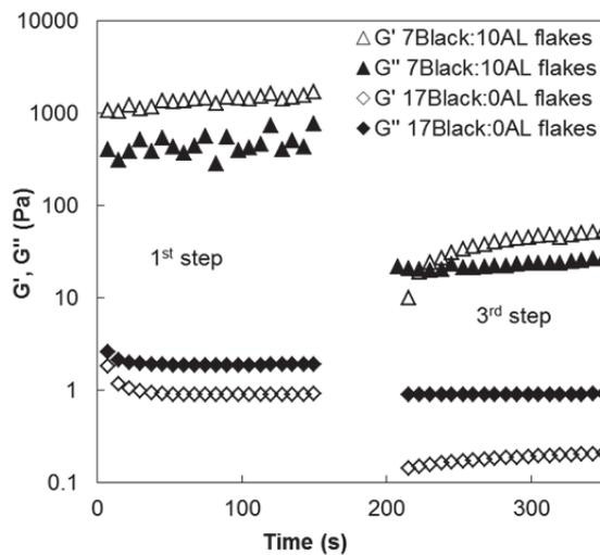
Figure 3. 3-step time tests for TISS paints: the effect of different ratio between black pigment and Al flakes.
