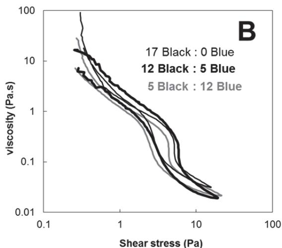
Figure 1. Flow curves for TISS paints: the effect of different ratio between A) black pigment and Al flakes; B) black and blue pigment.
