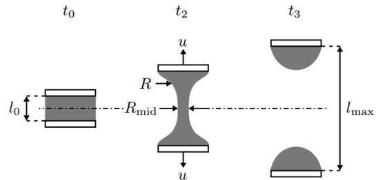
Figure 3 : Principle of extensional rheometry where a fluid element is placed between two plates at an initial distance,  $l_0$ . The plates move in opposite directions until a maximum distance  $l_{max}$  with a constant velocity  $u$ . A ligament establishes with a certain radius  $R$  and thins until break-up, where the mid-filament radius  $R_{mid}$  is observed.
