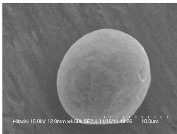
Figure 1 : A scanning electron microscopy image of an individual solder ball of a Sn-Ag-Cu alloy.
