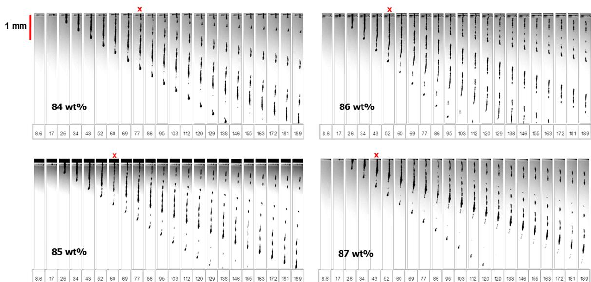
Figure 5 : Sequences of images showing the jetting of solder paste with 84–87 wt% using the same input ejection energy. Numbers below each image indicates time after droplet ejection in  $\mu$ s. The scale bar corresponds to 1 mm. The x symbol indicates complete pinch-off at the filament head.
