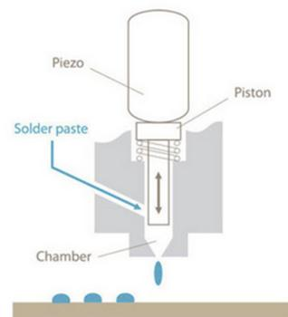
Figure 4 : Schematic of the jetting principle that is the impetus of this study.
