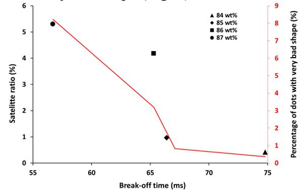
Figure 7 : Satellite ratio and percentage of dots with very bad shape when jetted onto substrate plotted against break-off time from FILBO measurement for solder pastes with 84 (▲), 85 (◆), 86 (■) and 87 (●) wt%.
