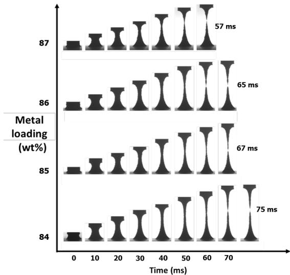
Figure 6 : Sequences of images showing the filament breakup of solder paste suspensions with 84, 85, 86 and 87 wt%.
