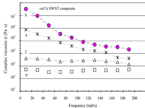
Figure 4: Viscosity of CNT-reinforced polyamide composite.
