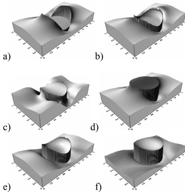
Figure 7: Nanotube pulling out at a range of interfacial fracture energy.
