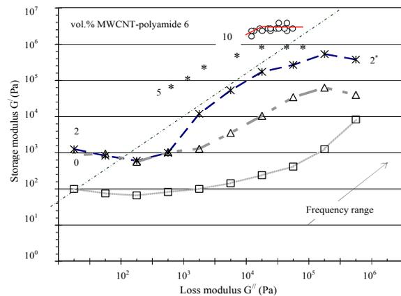
Figure 2. Comparison of storage and loss modulus due to CNT concentration.
