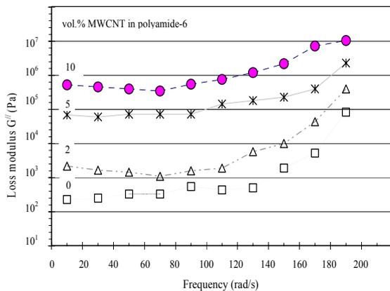
Figure 3: Loss modulus of CNT-reinforced polyamide composite at 300°C.
