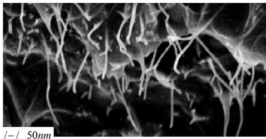
Figure 1. CNT-reinforced polyamide composite material.
