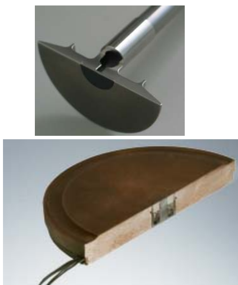
Figure 4. Cross-sectional views of prototypes of a Peltier lower plate (bottom) and an upper geometry (top). The solenoid system and the magnetic disc can be seen, respectively.
