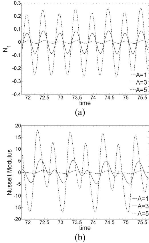
Figure 3. Time evolutions for increasing amplitudes at  $\text{Re}=0.3$ ,  $\text{We}=1$ ,  $\omega_r=0.55$ ,  $\text{Pe}=900$ ,  $\text{Br}=5$ ,  $\varpi=1.0$  and  $\varepsilon=1$  (a) First normal stress difference vs. time
