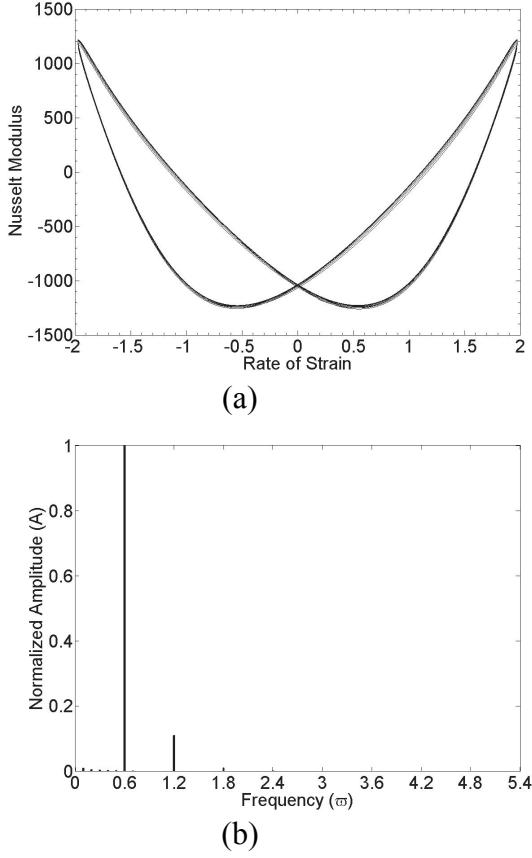
Figure 6.  $Re=1$ ,  $We=1$ ,  $\omega_r=0.55$ ,  $Pe=900$ ,  $Br=50$ ,  $\varpi=0.3$ ,  $\varepsilon=1$  and  $A=5$  (a) Lissajous of Nusselt modulus (b) Frequency spectrum.
