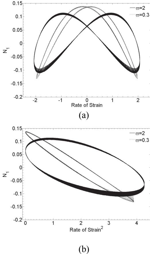
Figure 9. The first normal stress difference (N1) phase diagrams for  $Re=1$ ,  $We=1$ ,  $\omega_r=0.55$ ,  $Pe=900$ ,  $Br=50$ ,  $\epsilon=1$  and  $A=5$  at two different frequencies (a)  $N1$  vs. rate of strain (classic viscous Lissajous curve) (b)  $N1$  vs. rate of strain square.
