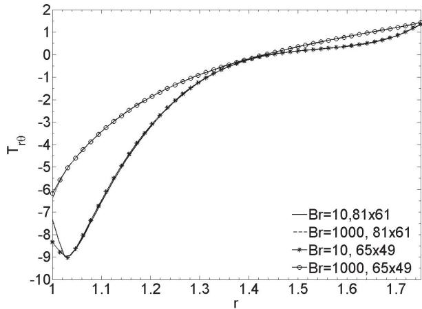
Figure 2. Comparison of shear stress distributions along radial direction (at  $\theta=0.2945$  rad.) for non-isothermal viscoelastic constant lid velocity case for two grid densities (81x61 and 65x49) and Brinkman values ( $Br=10, Br=1000$ ) at  $Re=0.5, We=1.0, \omega_r=0.4, \varepsilon=0.3, Pe=900$ .
