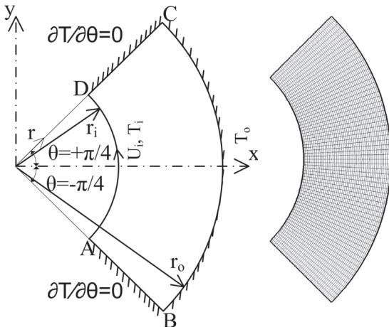
Figure 1. (a)Cavity Geometry<sup>12</sup>,
