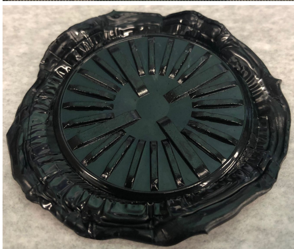
Figure 2. Test chamber of the MDR 2000 bi-conical moving die rheometer (top); rubber specimen after curing (bottom).
