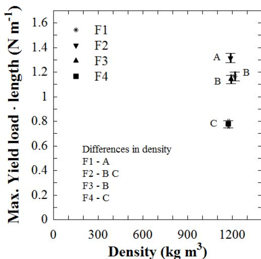
Figure 4: Max. yield load times length ( $\text{N m}^{-1}$ ) for the different sizes fractions. Different letters indicate significant differences ( $p < 0.05$ ). Letters beside the data points indicate significant differences in y - axis ( $p < 0.05$ ). Error bars represent the standard error of the mean ( $n = 40$ ).
