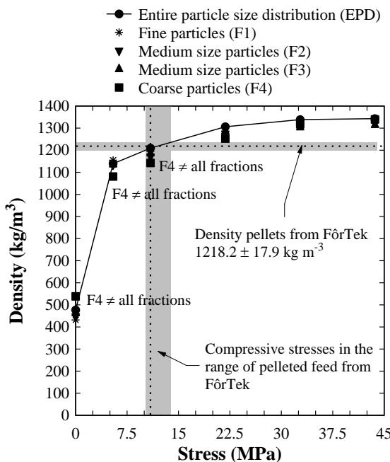
Figure 3: Compressibility plot of ground wheat grain and fractions. Data points are averages ( $n > 6$ ). Significant differences within the groups are indicated with symbol  $\neq$ . The grey bands indicate the range of densities and possible compressive stresses of the pellets manufactured in FörTek pilot plant. The dotted lines indicate the estimated pressure to produce pellets of similar density to the ones from FörTek.
