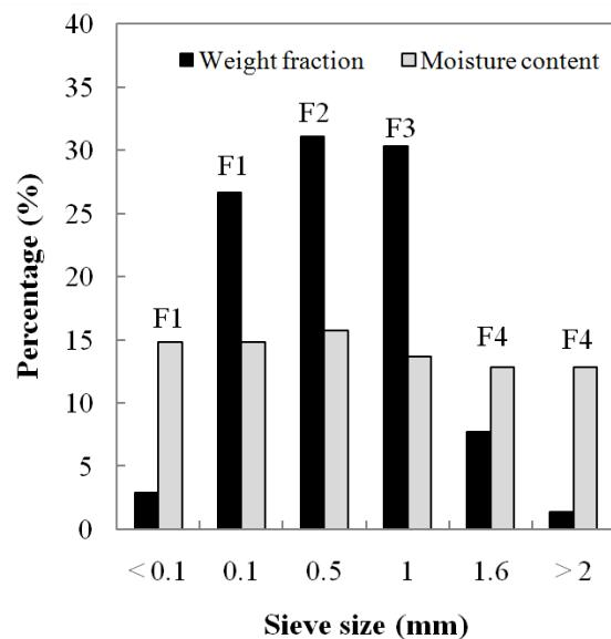
Figure 1: Particle size distribution and average moisture content of wheat grains ground in a hammer mill. F1, F2, F3 and F4 represent the size fractions used to manufacture the pellets.
