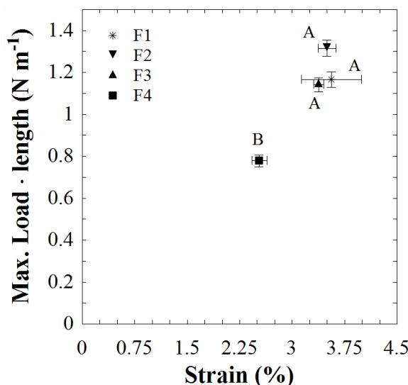
Figure 5: Max. yield load times length ( $\text{N m}^{-1}$ ) for the different size fractions showing the different levels of strain (%) at the moment of the main failure. Error bars represent the standard error of the mean ( $n = 40$ ).
