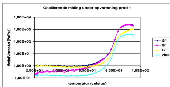
Figure 2. Temperature depended oscillatory measurement on the model fluid. Showing G', G'' and the viscosity.
