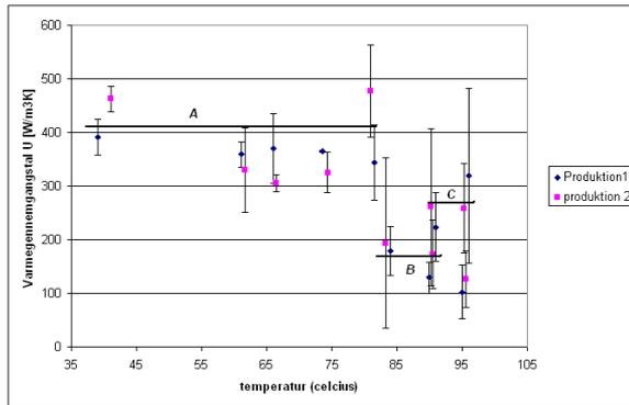
Figure 1. Overall heat transfer coefficient in the Push-Pull system depending on the temperature of the product
