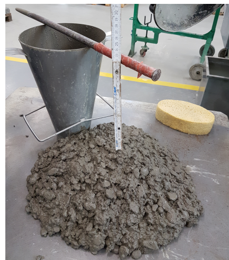
Figure 7. Slump test with Abrams’ cone on precast concrete
