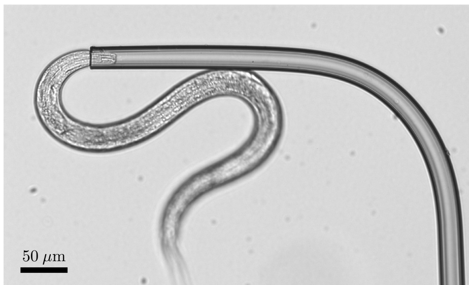
Figure 1. The material properties and swimming dynamics of the C. elegans nematode was directly measured using the micropipette deflection technique.
