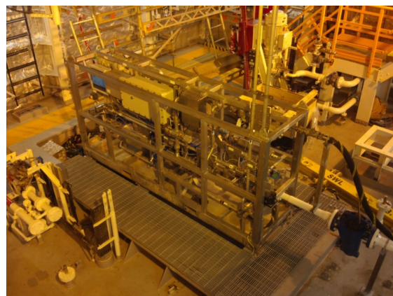
Figure 3. Offshore installation of the Pipe rheometer
