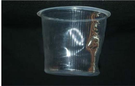
Fig.2. The warpage of a polymeric product during its application
