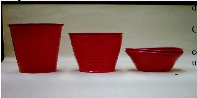
Fig.6. Comparison of warpage in PS products (**a**- initial product at T=298K without warpage, **b**- at T=353K with  $t_{pn} = 2$  sec., **c**- at T=353K without relaxation pause).
