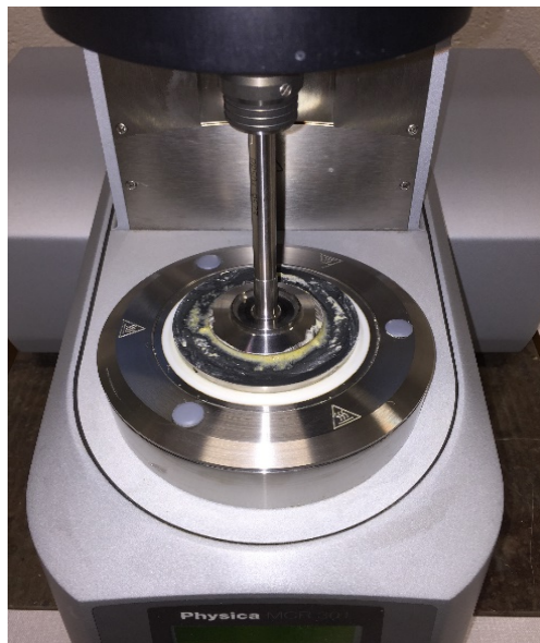
Figure 1: The plate-plate oscillation measuring system connected to a Physica MCR 301 rheometer.
