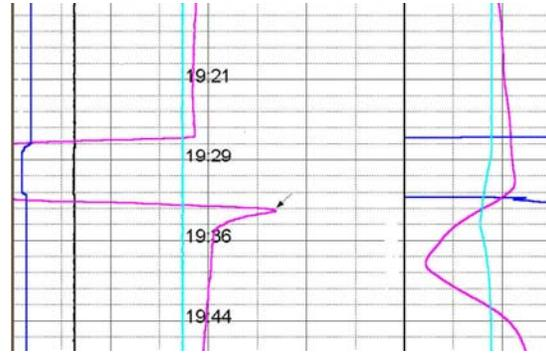
Figure 2. Gel peak after only 6 minutes rest - an increase of 417 psi
