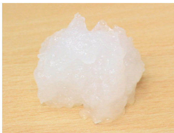
Figure 1. Photograph of MFC gel with a cellulose concentration of 2.2 weight-%.
