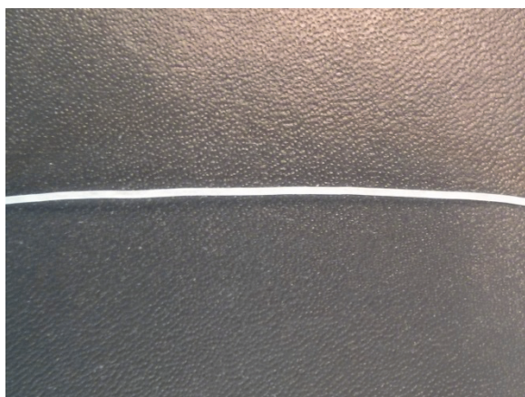
Figure 2. The Extruded fibre containing 30 weight-% MFC (nominal value).
