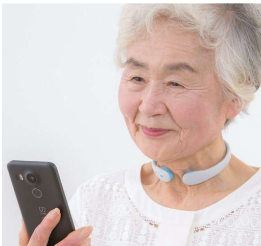
Figure 1: The swallowing sensor is placed on the patient's neck and records the sound during swallowing. It is connected to a mobile device where an app displays the swallow duration in real time and dysfunctionality can be detected directly.
