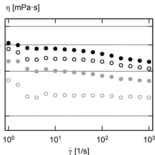
Figure 1. Viscosity curves of fermentation broth of ST-E (black) and ST-G (grey) with cells (closed) and cell-free (open).
