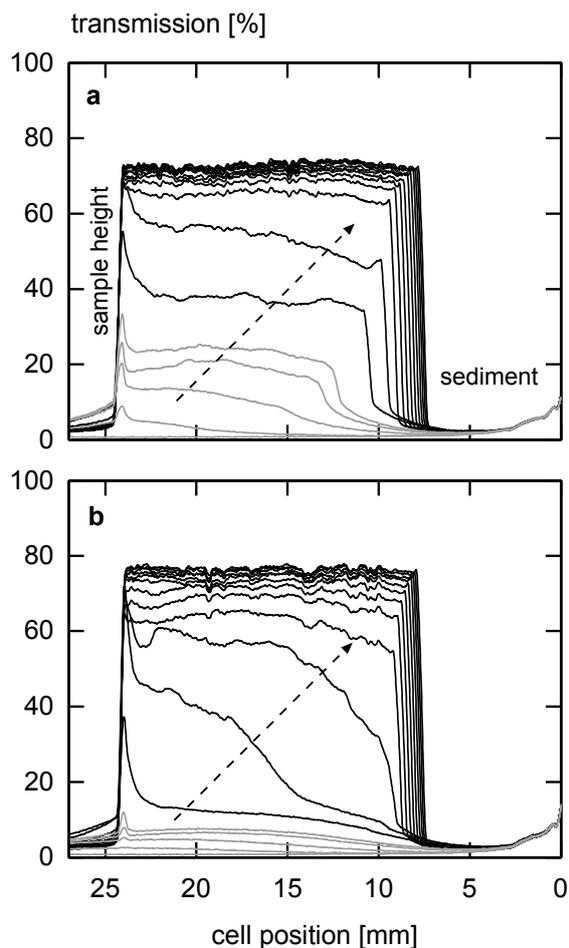
Figure 2. Transmission as function of cell position at selected time points during centrifugation of milk gels fermented with ST-E (a) and ST-G (b). 10 s (grey) and 100 s (black) intervals between transmission profiles. Arrow indicates time progress.
