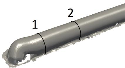
Figure 7. Scanned adhesive bead showing the two cross sections used for validation of the simulated beads.
