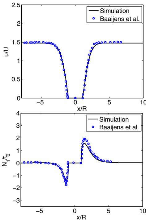
Figure 2. Streamwise velocity (top) and first normal stress difference (bottom) along the channel centerline for flow past the symmetrically confined cylinder.
