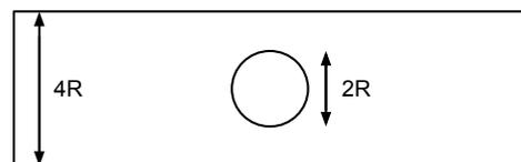
Figure 1. Symmetrically confined cylinder geometry.
