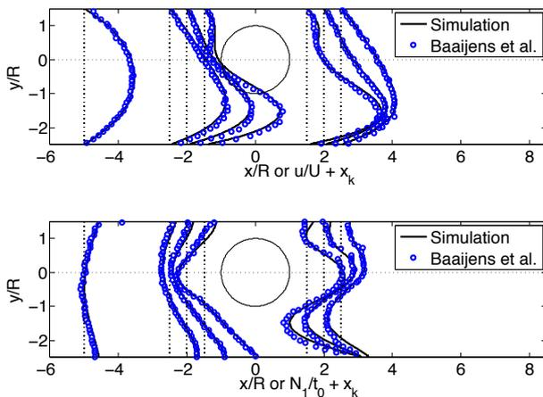
Figure 5. Streamwise velocity (top) and first normal stress difference (bottom) across the channel at different locations for flow past the asymmetrically confined cylinder.
