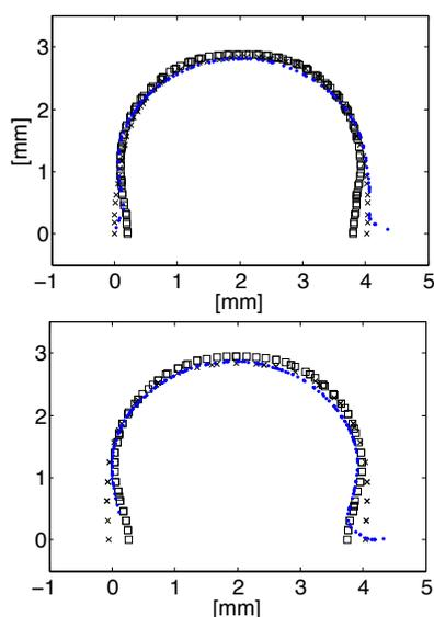
Figure 8. Cross section comparison at measurement position 1 (top) and 2 (bottom) between the bead simulated with 5 refinements ( $\circ$ ), 6 refinements ( $\square$ ) and the scanned bead ( $\bullet$ ).
