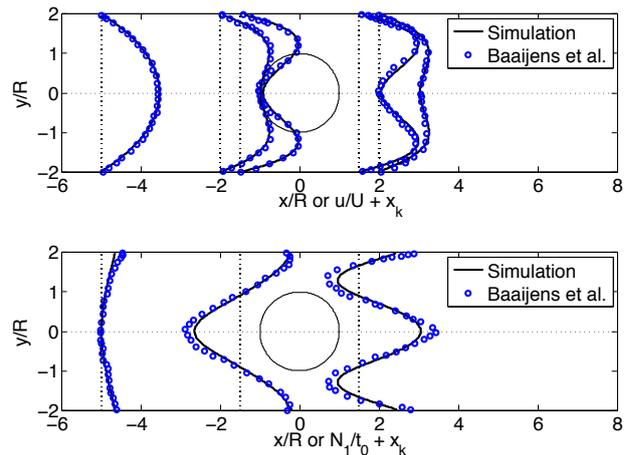
Figure 3. Streamwise velocity (top) and first normal stress difference (bottom) across the channel at different locations for flow past the symmetrically confined cylinder.
