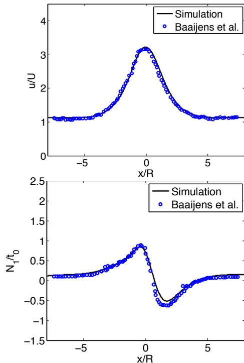
Figure 4. Streamwise velocity (top) and first normal stress difference (bottom) along the channel centerline for flow past the asymmetrically confined cylinder.
