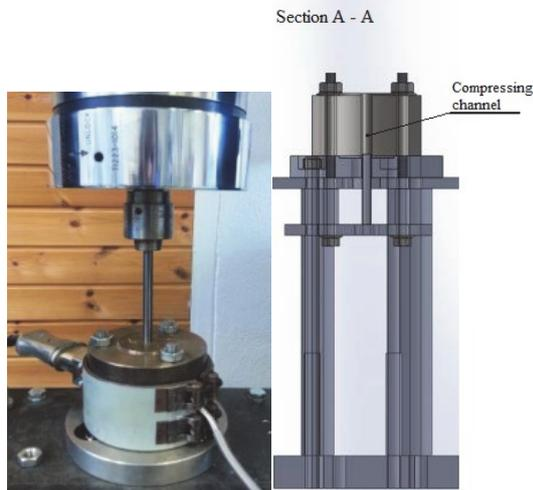
Figure 1. Single pellet press unit: picture of the equipment (left) and section view A-A (right).
