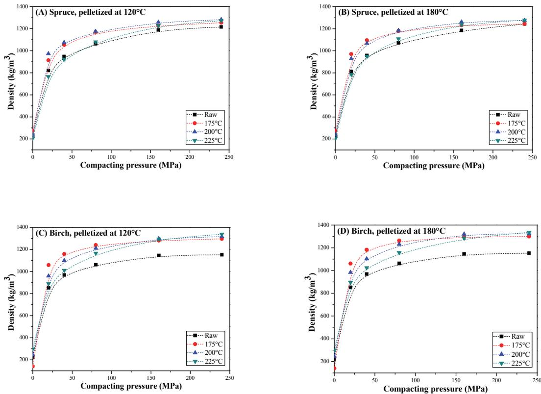
Figure 4. Density of pellets made at different pelletizing pressures and temperatures.
