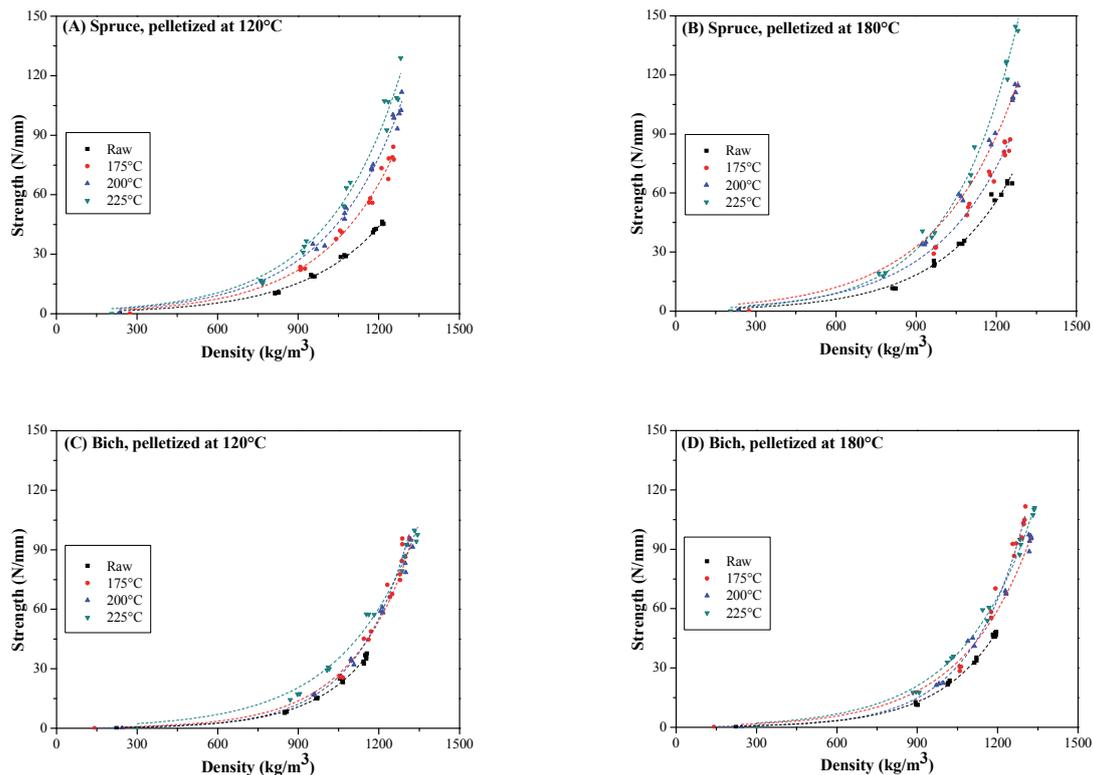
Figure 6. Relationship between density and strength of pellets produced at different compacting temperatures.
