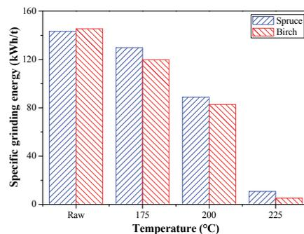
Figure 2. Specific grinding energy of raw and wet-torrefied forest residues.
