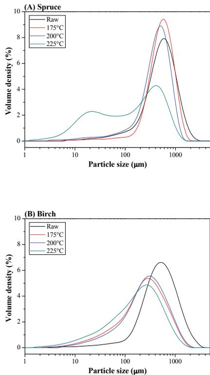
Figure 3. Particle size distribution of ground (A) spruce and (B) birch.
